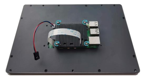
8. Plug the power cord into the corresponding 40-Pin on the Raspberry Pi 5.
